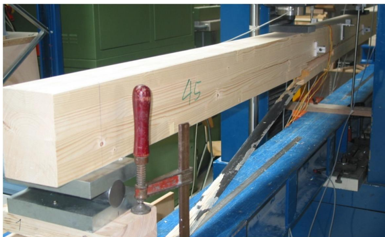
Figure 92: Specimen 45 after complete failure and unloading. The delamination of the CFRP-lamella was most likely forced by the failure of the timber.
