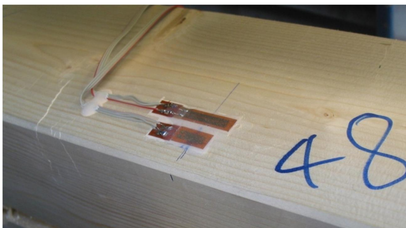
Figure 84: Specimen 48 after complete failure and unloading. The crushing is clearly visible on the left side of the image. In the centre, the two strain gauges are visible (the shorter one has a measuring grid of 10 by 6mm and the longer one, a grid of 20 by 0.7mm).
